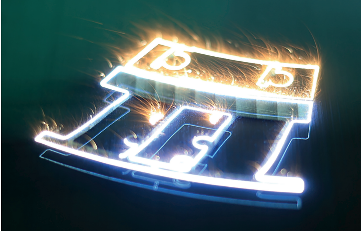
Exposure of an inlet guide vane (IGV) in the LPBF process.
