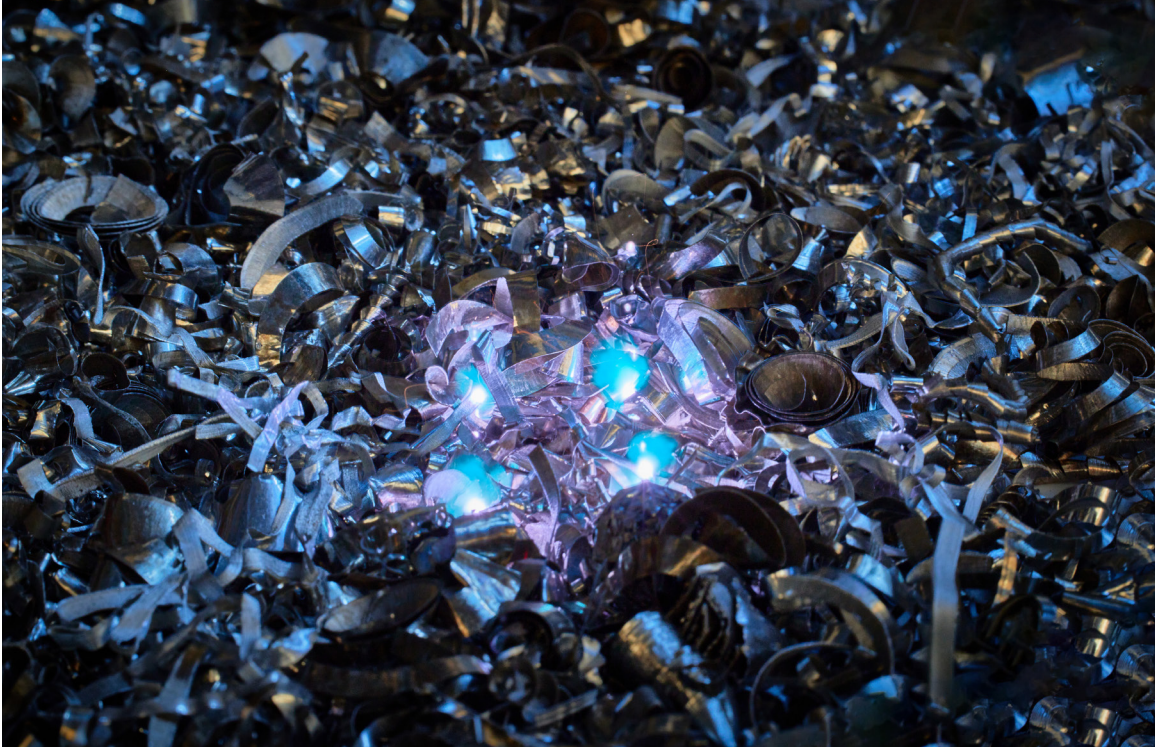
1 LIBS measurements of steel chips.
