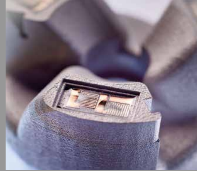
Sensing tool of the future: milling head with integrated sensors for temperature and pressure measurement.
