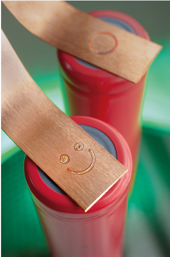
Picture 1: Laser-Based Tape- Automated Bonding (LaserTAB) for the welding of battery cells. © Fraunhofer ILT, Aachen, Germany.
