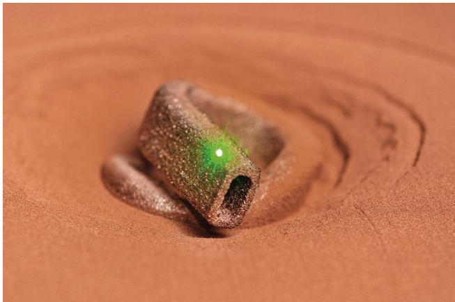
Picture 2: “SLM in green”: the new process should allow 3D printing of pure copper components. © Fraunhofer ILT, Aachen, Germany.
