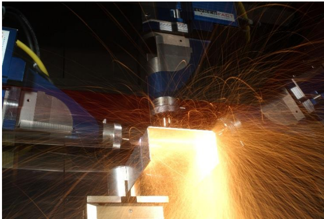
Image 1: Laser combi-head for cutting and joining as well as additive manufacturing by means of laser metal deposition.
