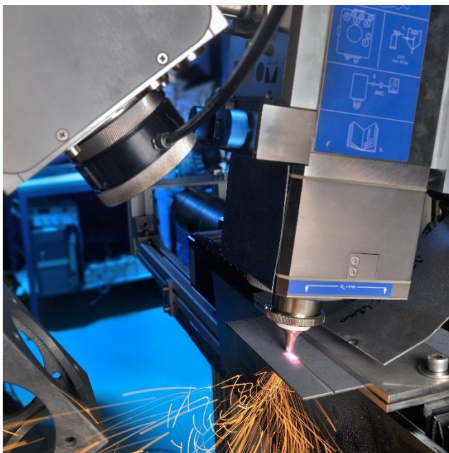
Image 2: Laser cutting with subsequent laser for heat treatment.
