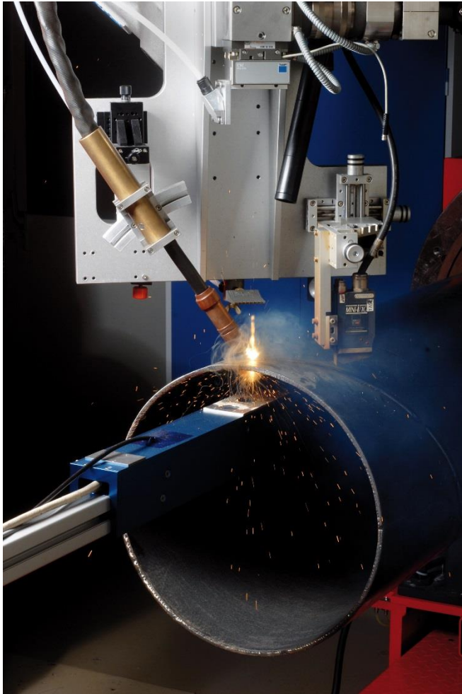
Image 2: Process monitoring and adaptive control for laser MSG hybrid welding. © Fraunhofer ILT, Aachen, Germany.
