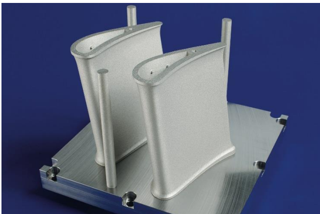
Image 1: Individually manufactured segments of the guide vanes for the modular process chain (material: Inconel® 718).
