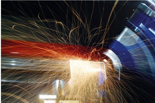
Picture 1: The laser combi-head cuts, measures and welds metallic assemblies without tool change. © Laserfact.
