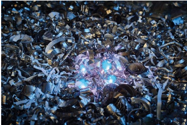
Image 3: Analysis of metal scrap by laser-induced breakdown spectroscopy LIBS. © Fraunhofer ILT, Aachen, Germany / Volker Lannert.
