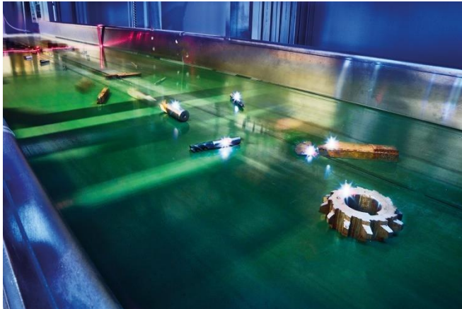
Image 1: Laser-induced breakdown spectroscopy LIBS detects valuable alloys in scrap metal, which robots separate by type. The process creates the basis for closed material cycles without downcycling. © Fraunhofer ILT, Aachen, Germany / Volker Lannert.
