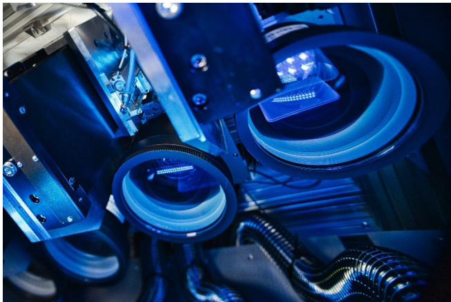
Image 4: The multi-beam multiscanner optics developed by Pulsar Photonics is designed to increase the throughput of battery cell production with the help of 24 partial beams. It is used in a facility of the Battery Center at Fraunhofer ILT.
