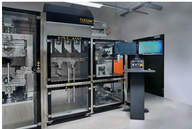
Image 2: Since 2021, laser processes for battery production have been researched at Fraunhofer ILT in a dedicated battery center. Here in the picture, the facility with the multi-beam optics for laser processing. In the next step, Pulsar Photonics wants to bring the optics developed for the NextGenBat project to series maturity - ideally with industrial partners. © Fraunhofer ILT, Aachen, Germany.
