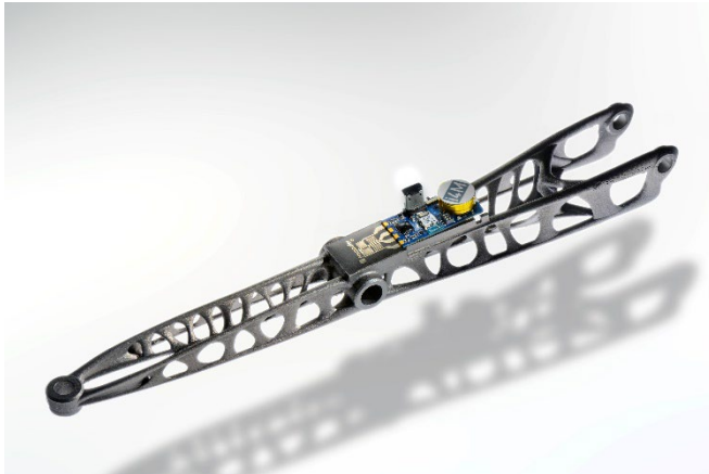
Image 1: The transverse link with imprinted force sensor measures the stresses acting in the application at any time and registers the smallest cracks that occur before a defect occurs. © Fraunhofer ILT, Aachen, Germany.
