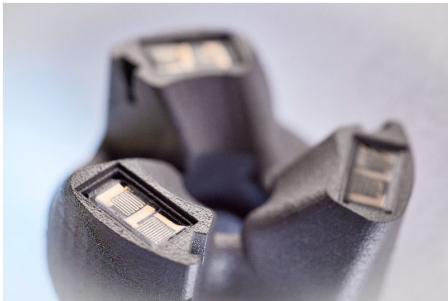
Image 2a: Strain gauges were integrated into a cutter head during the printing process. Before: The LPBF printing process is interrupted and the strain gauges, which were also printed, are integrated. © Fraunhofer ILT, Aachen, Germany.
