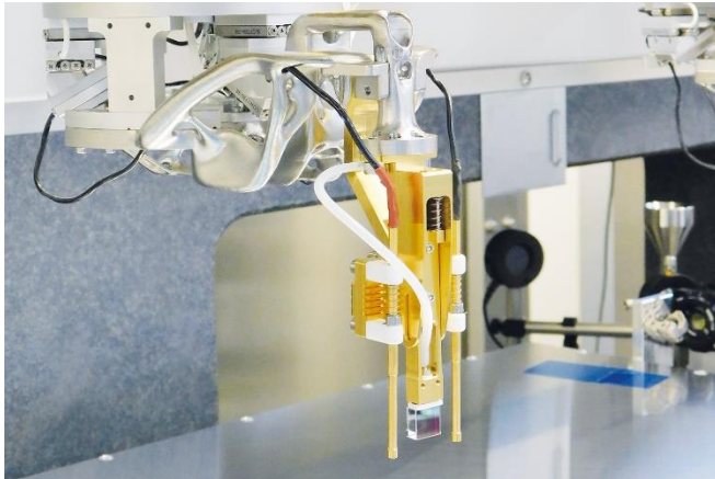
Figure 1: The gripper arm – the central tool for the high-precision alignment of space components – consists of a static and a moving part. © Fraunhofer ILT, Aachen, Germany.
